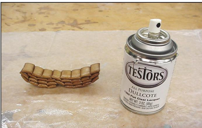
A coating of Testors Dullcote Lacquer was applied, which gave the assembly a rich color, and sealed in the chalk.
